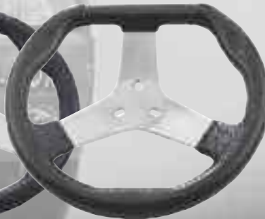
688 Kart Model "D" Shape Wheel, Molded Polyurethane Grip with a Leather Grained Finish. Silver Anodized Aluminum Spokes. 11 1/4" Diameter, 1 1/4" Dish.
