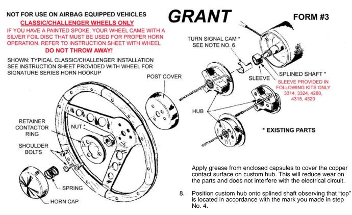
ATTN: TOYOTA (HUB NO. 10179) AND HONDA/ACURA VEHICLES (HUB NO. 10069). THESE HUBS ARE DESIGNED TO FIT ONTO THE SHAFT VERY TIGHTLY AND BE DRAWN DOWN BY TIGHTENING THE SHAFT NUT.
