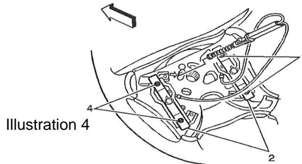
2. Remove the horn switch assembly by loosening the 4 T-30 Torx screws (numbers 1 and 4) holding the contact plates to the steering wheel and remove this entire mechanism (2) from the wheel. **Note orientation** (wires at the top of the switch mechanism) so you do not reinstall upside down. See Illustration 4 above.
