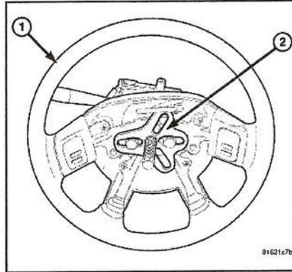
2. Taking care to not pull on any of the wiring coming out of the column; simply feed the wires back thru the hole in the wheel and remove the wheel from the column. Again, do not turn the plastic clockspring mechanism now or at any time during the installation.
